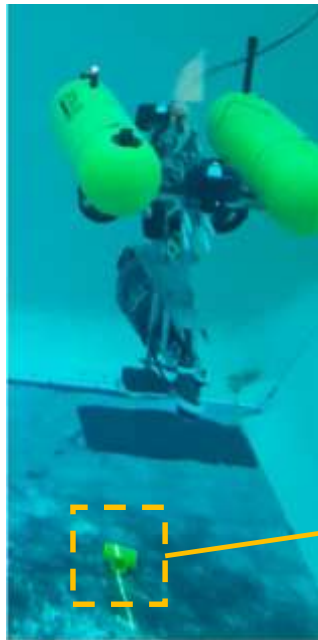
Girona 500 AUV with the laser scanner.
