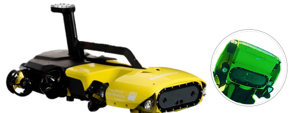
Fig. 1: The RangerBot AUV is a vision-only robot with two stereo camera pairs for performing navigation, obstacle avoidance and science/management tasks. (Inset) the downward facing stereo camera pair and LEDs.
