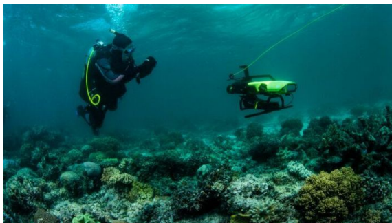
Fig. 11: A RangerBot AUV with the first prototype coral larvae delivery system during reseedling trials on the Great Barrier Reef in December 2018.
