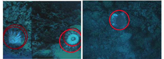
Fig. 9: Example of real-time multi-COTS detector output. (Left) Detector results before a non-maxima suppression stage where multiple over labelling detections are merged together. (Right) Improved overall COTS segmentation.
