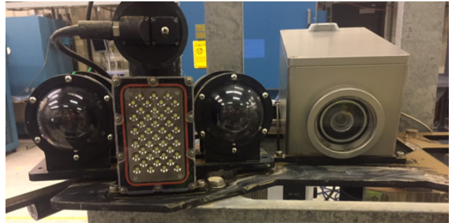
Fig. 1. The vision system. The two cameras with dome ports are on the left and middle. The projector is on the right side of the image.
