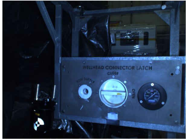
Fig. 3. This is the example task panel used in testing the quality of 3D reconstruction methods.
