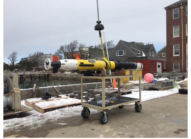
Fig. 2: Snoopy AUV, equipped with broadband echosounder, nitrate sensor, and other environmental/navigation sensors, preparing for deployment in March 2019 at Woods Hole Oceanographic Institution.
